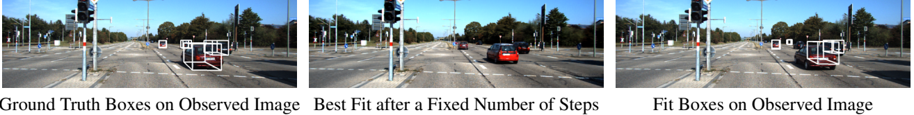
Figure 12: 3D Object Detection via Inverse Rendering. For the observed image on the left, the 3D object detection results in the rendering presented in the middle after a fixed number of iteration steps. The poses and dimensions for all objects from the corresponding scene graph are drawn as 3D bounding boxes on the right.
