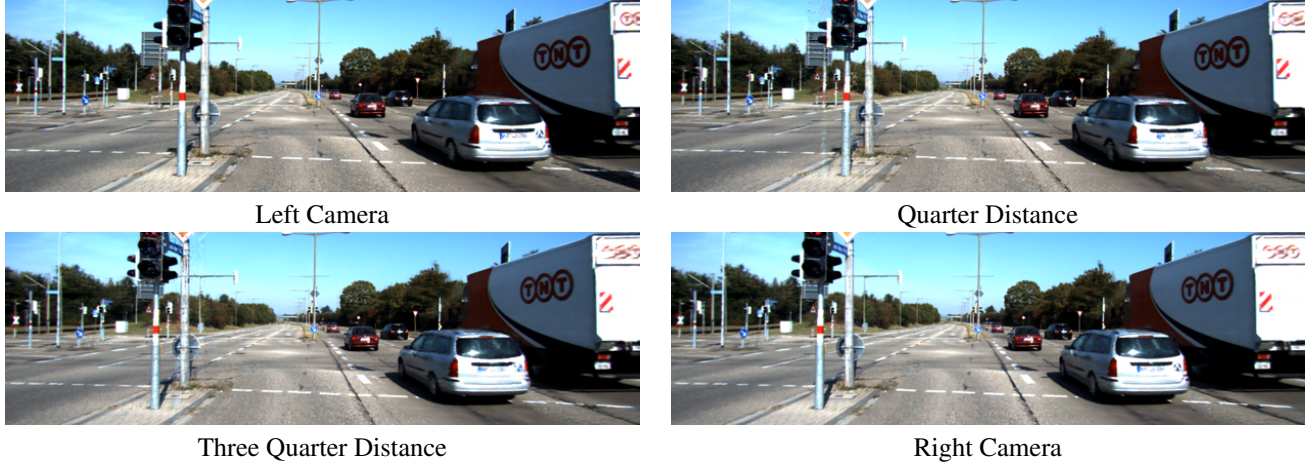
Figure 6: Demonstration of view interpolation of the camera position. We translate the camera pose from the left camera to the right camera of the stereo camera setup from a KITTI sequence [2].
