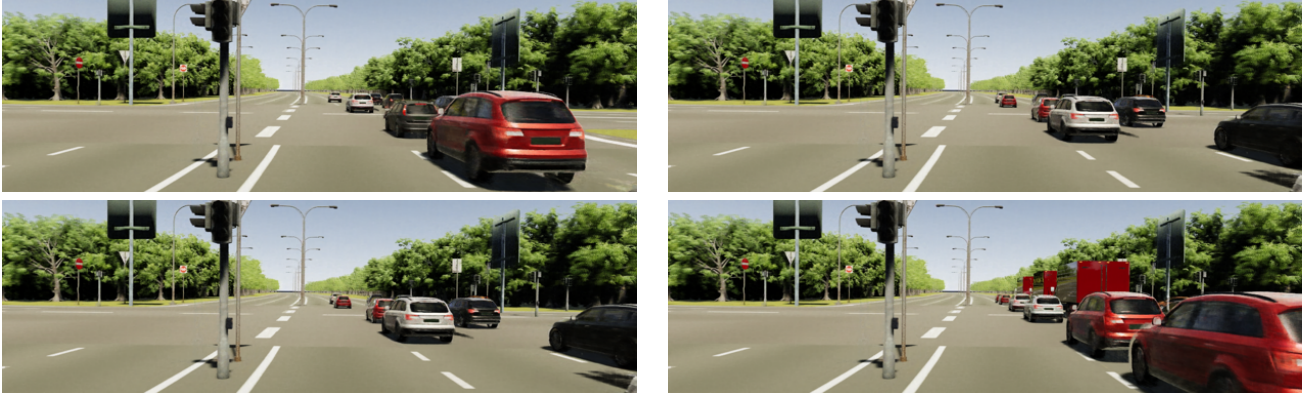
Figure 4: Renderings from Novel Scene Graphs. Randomly sampled scene graphs using the nodes of a scene from Virtual KITTI2 [1] demonstrates the neural scene graph method applied to synthetic data.
