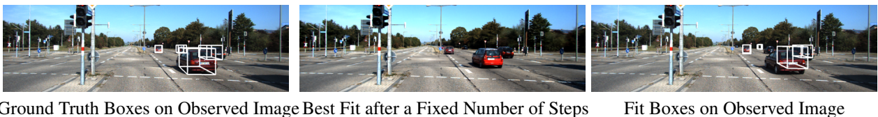
Figure 13: 3D Object Detection via Inverse Rendering. For the observed image on the left, the 3D object detection results in the rendering presented in the middle after a fixed number of iteration steps. The poses and dimensions for all objects from the corresponding scene graph are drawn as 3D bounding boxes on the right.
